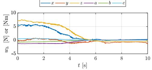
Fig. 4. Force guidance rendered by the Master Tool Manipulator during the haptic-guided needle grasping experiment.
