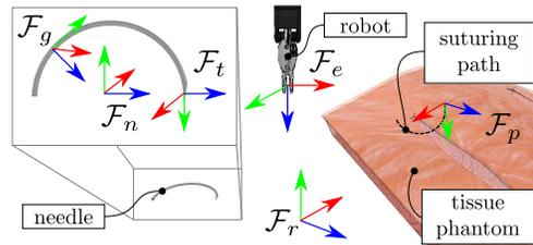
Fig. 1. Main reference frames and needle tip path (dashed black curve) for a single-stitch suturing task.
