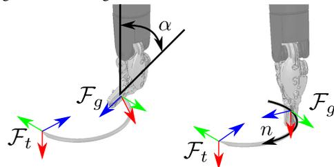
Fig. 2. Grasp parameterization by  $\alpha$  (angle around the needle tangent) and  $n$  (needle curvilinear abscissa) [2], [3].
